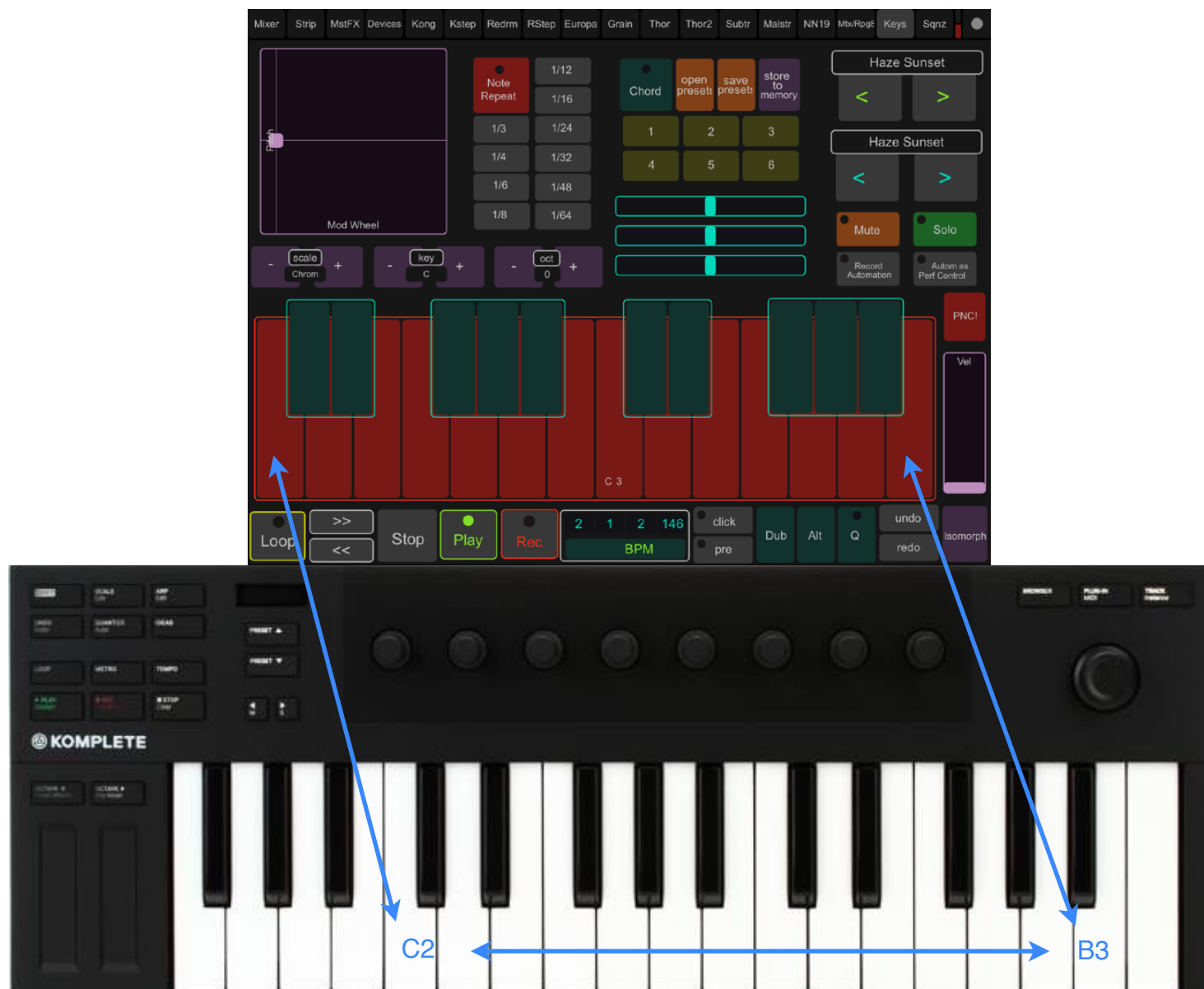
Setting up an external MIDI controller
