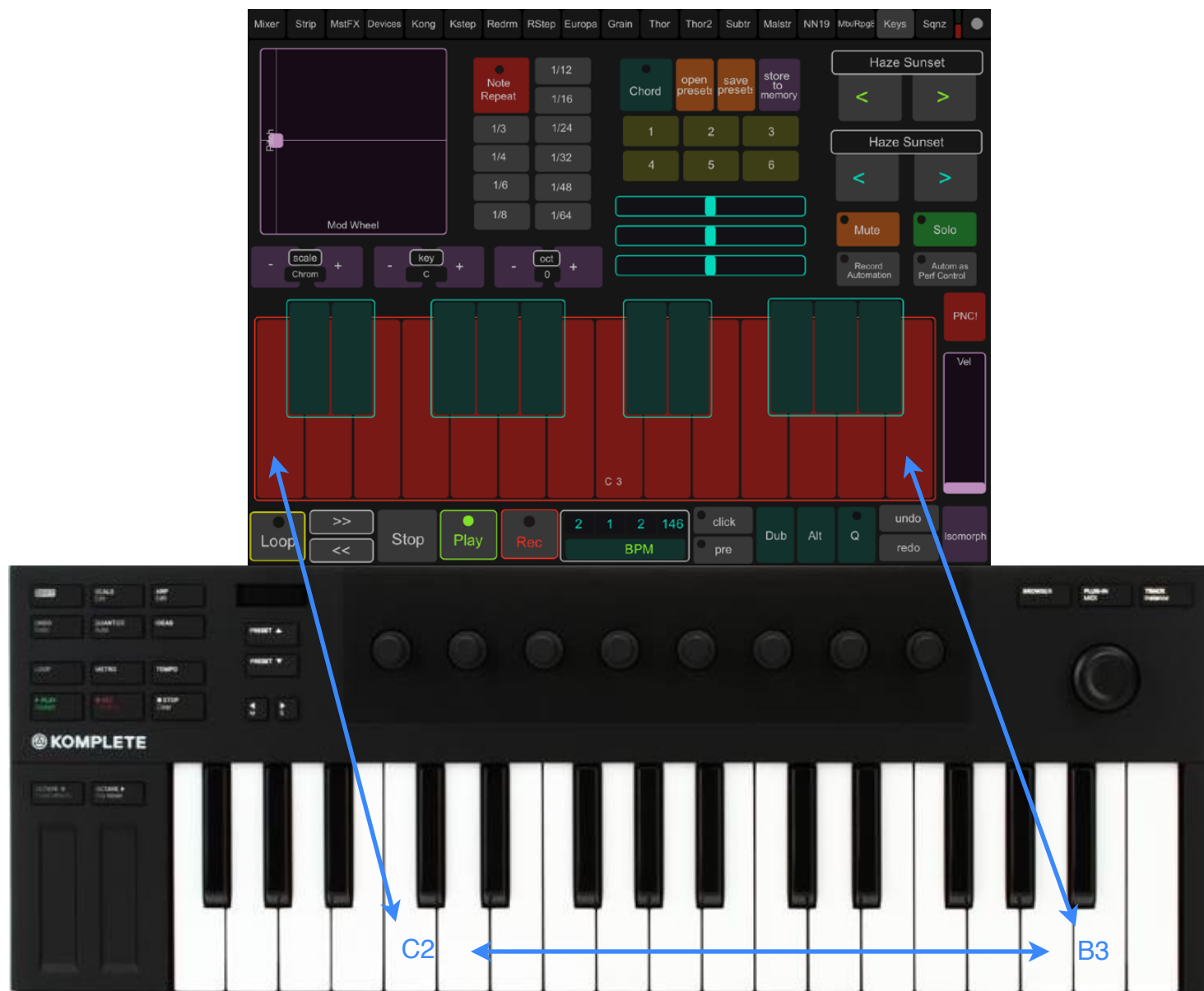
Setting up an external MIDI controller
