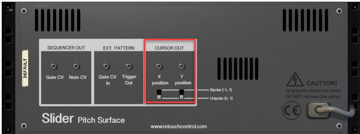
X and Y position CV outlets & polarity switches
