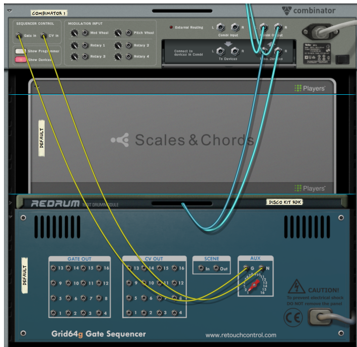
Connect the AUX Gate and Note to the inputs of a combinator
